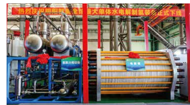
In October 2022, the alkaline water electrolysis hydrogen production equipment with the world's largest single hydrogen production capacity of 1,500-2,500Nm 3 /h at that time came off the production line.
